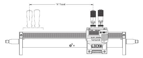
Figure 2. Typical dimensions for Maury slide screw tuners. See the Available Models table for model-specific dimensions ("A" reference).
